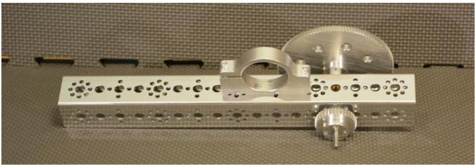
Step 4: assembly from step 3, 288mm channel (1), 144mm angle (1), 1/2" socket head cap screws (4), and keps nuts (4). The second picture shows the completed step.
