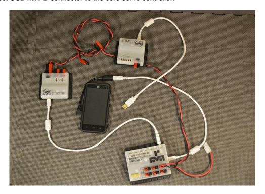
Step 13: Connect USB A connector to any of the remaining USB ports on the core power distribution module.
