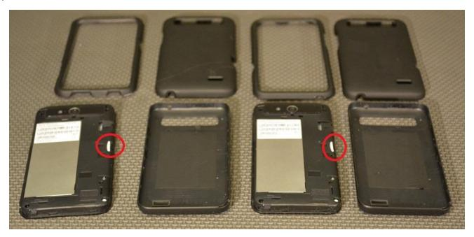
Step 4: Let the spring gently push the SIM cards from the phones. Pushing the SIM cards activate the spring mechanisms; releasing pressure allows the springs to push the SIM cards out of the phones.
