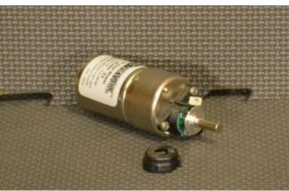
Step 4: snap the encoder cover onto the motor encoder.
