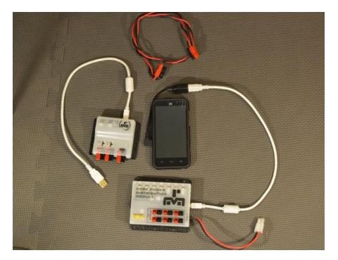
Step 8: Connect USB A connector to any of the remaining USB ports on the core power distribution module.
