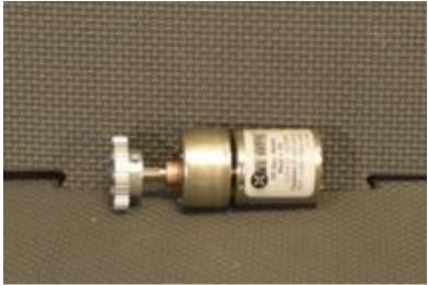
Step 9: Install the motor in the motor mount on the Robot tower. Rotate the motor in the mount to mesh the gears. Do not mesh the gear too tight or the motor will bind. Do not mesh the gears too loose or the teeth will slip.
