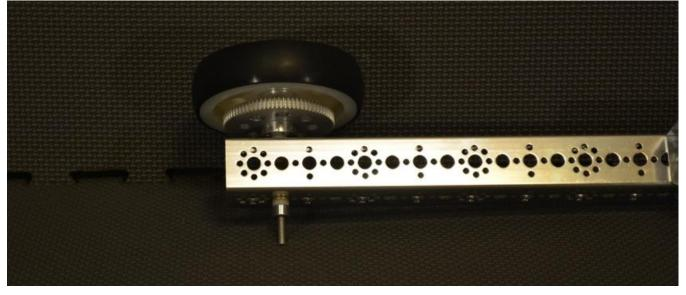
Step 3: assembly from step 2, omni wheel assembly (1), 1/8" axle spacer (2), 3/8" axle spacer, axle collar (2), bronze bushing (2), and axle (1). Note: assembly order is axle collar, 1/8" spacer, omni wheel assembly, 1/8" spacer, bronze bushing, channel, bronze bushing, 3/8" spacer, and axle collar. The second picture shows the completed step.
