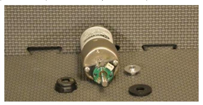
Step 3: install the encoder disk on the motor shaft using the provided spacer tool. The first photo shows the spacer tool on the motor shaft setting the disk position. The second photo shows it without the spacer tool.
