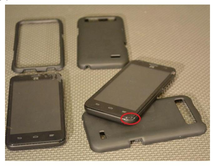
Step 3: The batteries are on the left and the SIM cards (circled) on the right. Gently push the SIM card INTO the phone.
