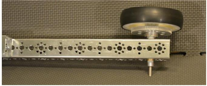
Step 3: assembly from step 2, omni wheel assembly (1), 1/8" axle spacer (2), 3/8" axle spacer, axle collar (2), bronze bushing (2), and axle (1). Note: assembly order is axle collar, 1/8" spacer, omni wheel assembly, 1/8" spacer, bronze bushing, channel, bronze bushing, 3/8" spacer, and axle collar. The second picture shows the completed step.
