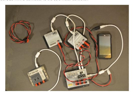
Step 17: Connect USB A connector to any of the remaining USB ports on the core power distribution module.
