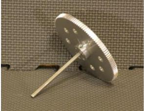
Step 2: assembly from step 1, 288mm channel, 3/8" axle spacer (1), bronze bushing (2), 1/8" ax axle el spacer (1), 40-tooth gear (1), axle hub (1), and button head cap screws (4). The second picture shows the completed step. Note the order on the axle. 120-tooth gear, axle hub, 3/8" axle spacer, bronze bushing, channel, bronze bushing, 1/8" spacer, 40-tooth gear, and axle hub.
