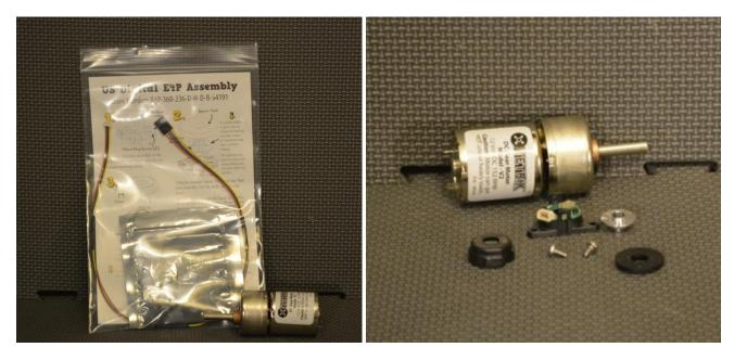
Step 2: install the encoder printed circuit board assembly to the motor with the provided screws.
