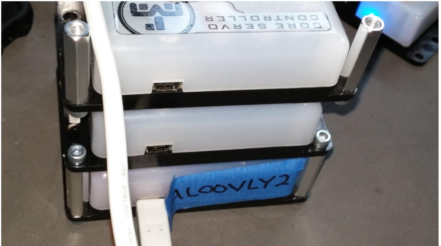
3: Label each component's Serial Number. Here, the Servo Controller's Serial Number is labeled.
