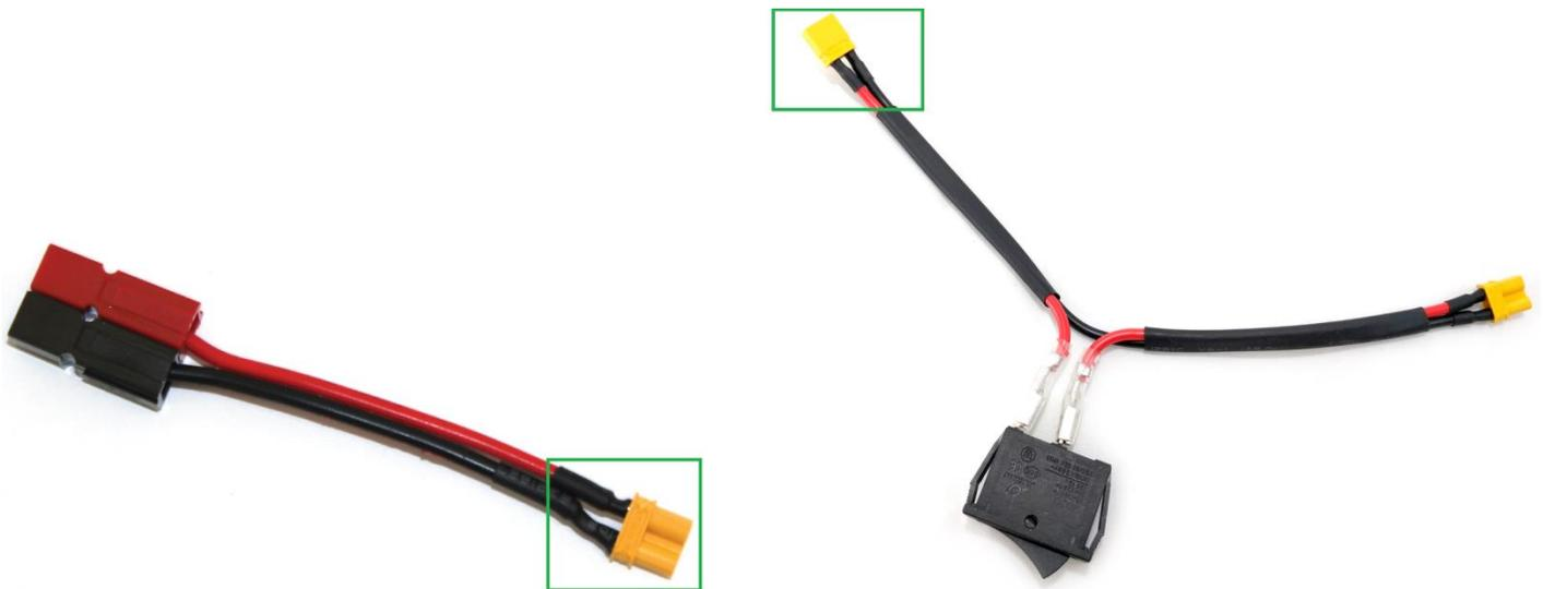
Step 4: Connect the Battery to the Switch Adapter Cable chassis
