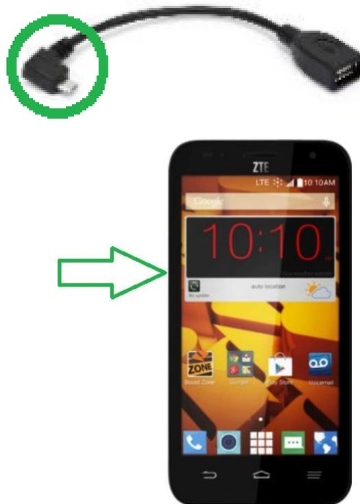
Step 3: Connect the USB Cable to the Micro USB OTG Adapter Cable chassis, micro USB OTG adapter cable (1)
