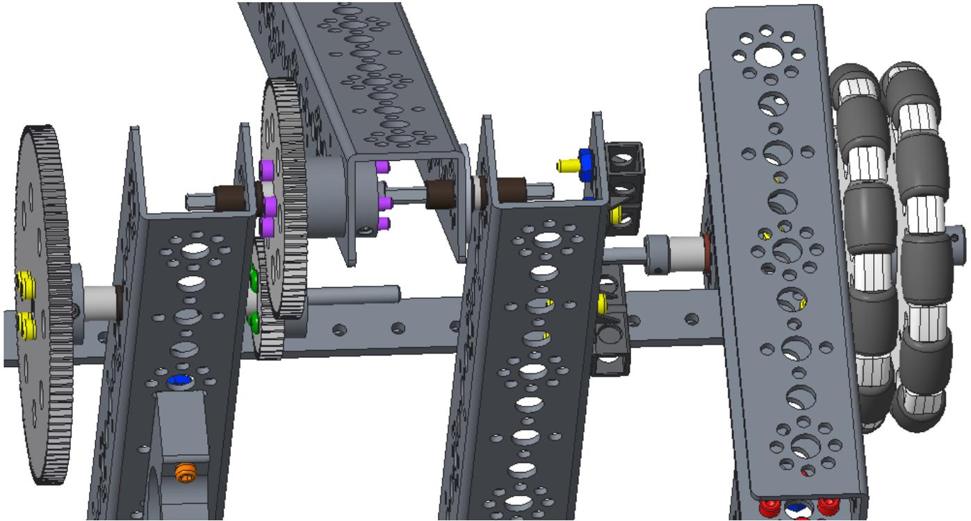
**Step 7: Adding the Expansion Hub Support Brackets**
