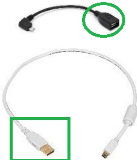
Step 4: Connect the Micro USB OTG Adapter Cable to the Expansion Hub chassis
